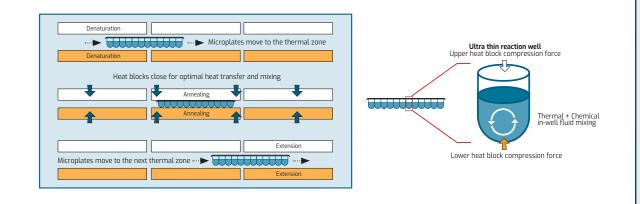
NextGenPCR® technology uses SBS-format microplates. The plates are sealed with heat seals creating wells that can be compressed by the heat blocks in each temperature zone. Compression has several beneficial effects to the speed and precision of the PCR reaction.
