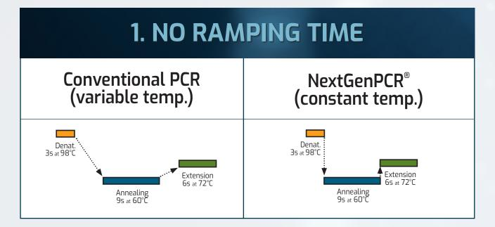
In conventional PCR, a microplate is placed in a machine that heats and cools using Peltier elements. Peltier technology is used to heat and cool a metal block, which in turn heats and cools the microplate and its content. Nearly all thermal cyclers use Peltier technology, despite its lack of speed.
